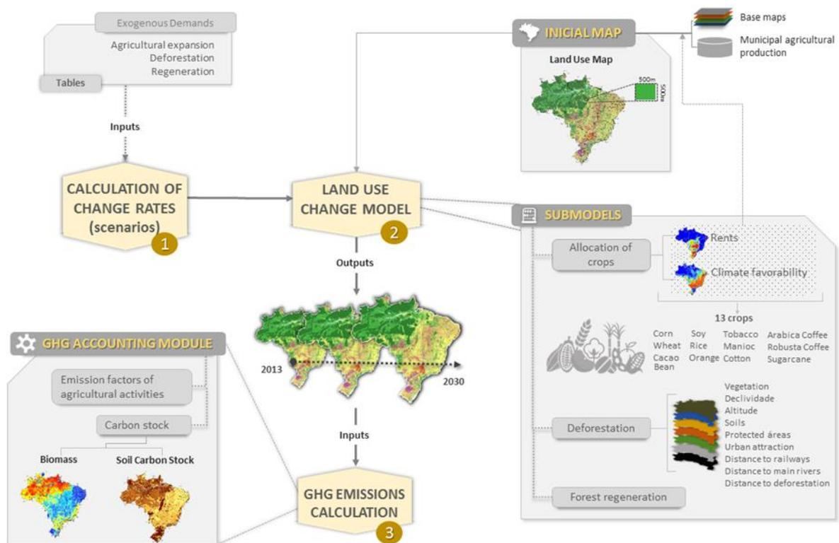
Figure 38: modelling framework developed for the Brazil case-study. Steps: 1) Projection of EU demand for ethanol to 2030 (with MAGNET model); projections of the other crops' growth to 2030 (MAPA, 2017). 2) Allocation of all productive croplands (with OTIMIZAGRO model) and calculation of land use changes. 3) Estimation of GHG emission from LULUCF and farming (with OTIMIZAGRO model).
